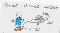
A simple desktop apparatus keeps coffee hot all day. Solar panel is located near a window; wire runs to pad. Specification
